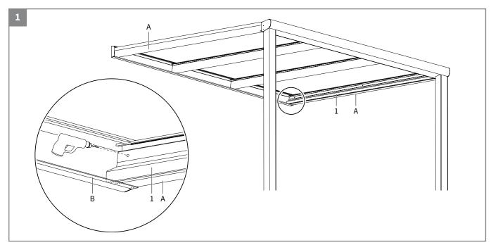
With this 3 meters wide conservatory blind the side guides (1) are mounted against the outer veranda beams (A).
