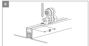
Tighten the running wheel with an Allen key. Size (B) depends on the position of the side guides. With the 3 meters version the size is 50 mm.
