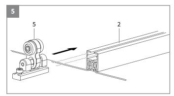
Slide the running wheels (5) into the stiffeners (2), on both sides. Mind the position of the allen bolt.
