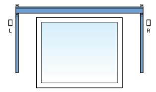
Determine the control side always seen from the outside. Pay extra attention if electrical control is desired. If the output side of the cable is on the left (front view), the inside control needs to be on the right.
