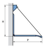
The bigger the projection, the bigger the effect of the drop-arm awning. Only standard sizes are possible: 100, 115, 135 or 150 cm.
