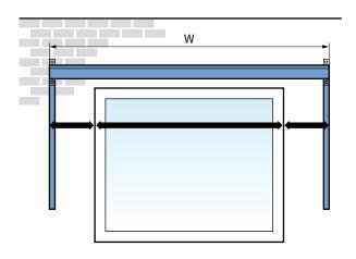
It is advisable to measure the drop-arm awning as wide as possible. We advise this with regard to the turning of the sun and to prevent possible light incidence at the sides of the window. If possible, provide at least 50 to 100 centimeters overlap. It will not be a problem if you, for example, can only provide a 30 centimeter overlap.
