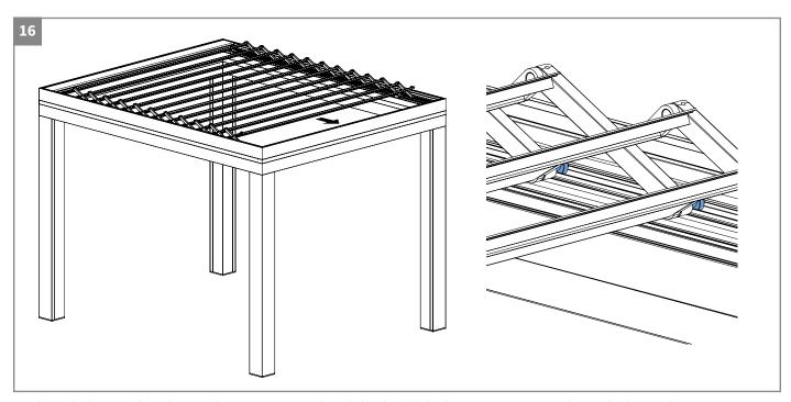
• Close the louvered roof using the remote control and check if all the bearings run correctly inside the guides.
