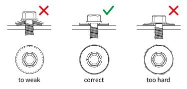
diameter 4,8 mm rotation speed 1.800 tr/min torquemoment 25 kg
