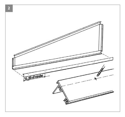
Provide the 4 covering profiles with Ø 4 mm holes. The long covering profiles 6 holes, 10 cm. From the ends and the short covering profiles 2 holes Ø 4 mm.
