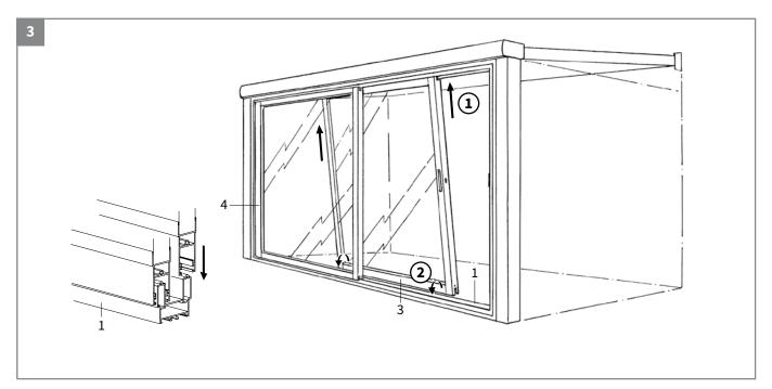
Install the sliding window part (3) to the rail (1) (inside rail).
