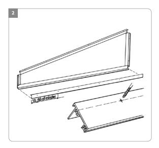
Provide the 4 covering profiles with Ø 4 mm holes.
