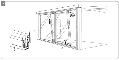
Install the sliding window part (3) to the rail (1) (inside rail). **Attention!** Wheels underneath.
