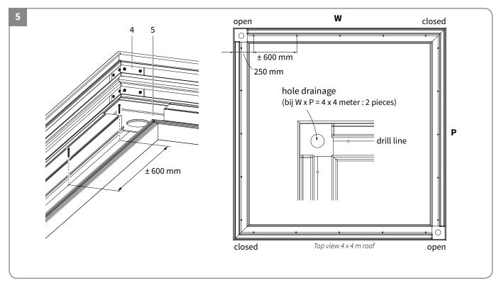
Tighten the gutter on the casing profile using screws on the drill line. Make sure that the gutter fits well on the casing profile.
