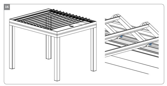
• Close the louvered roof using the remote control and check if all the bearings run correctly inside the guides.
