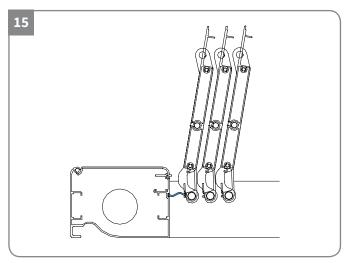
Check the seal between the slat assembly and the motor box.
