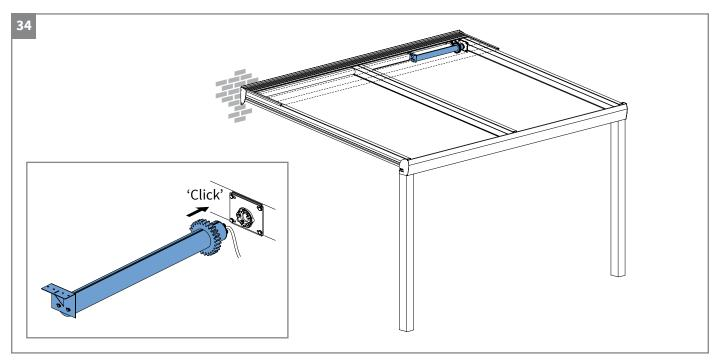
• Place the engine unit. Click the tube on the support of the engine plate. The sprockets now stack inside each other.
