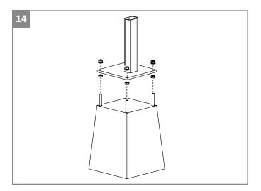
• Install the foot plates to the concrete bases.
