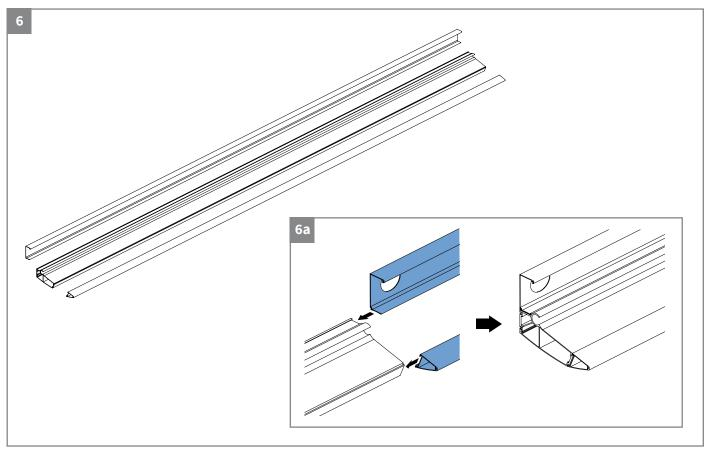
• Slide the three gutter profiles into each other.
