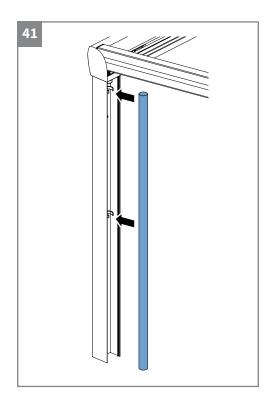
For each pipe, two clamp supports Ø 50 are needed.
