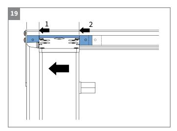
• Slide the connection pieces and the beam tightly to the end cap.
