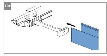
• Slide the upright over the connection piece all the way up to the gutter.
