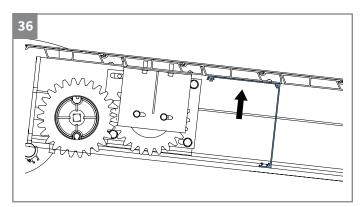
• Screw the corner profiles to the bottomside of the third roof plate in the pre-drilled installation holes.
