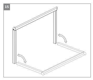
• Straighten the uprights with the gutter.
