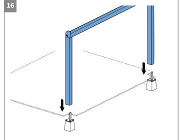
• Place the uprights over the installation feet and fixate levelled. The foundation blocks have welded threated ends with each two nuts, thus the uprights can be adjusted in height.
