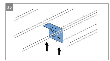
• Screw the engine unit from the lower side to the roof plate in the pre-drilled installation holes. (The position of the screw hole can variate regarding the drawing.)
