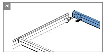
• Slide the side beam and the outermost connection piece against it.
