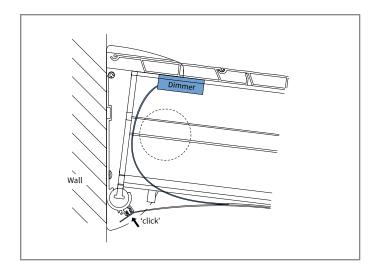
• As an option, the dimmer can be installed under the first roof can be mounted under the first roof plate.
