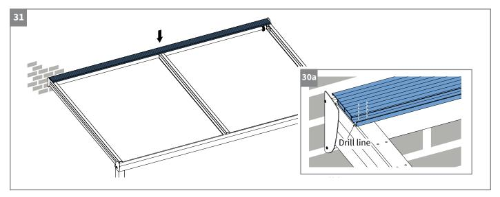
• Place the first roof plate and screw it to the beams.
