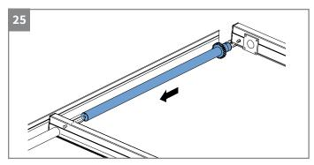
• Place the drive shaft against the centre beam. To make space, slide the side beam and the connection piece to the side.
