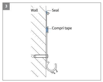
• Seal the complete edge of the wall profile at the top.
