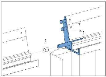
• Slide the connectors into the gutter profile and secure.
