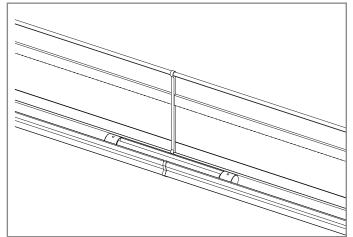
• Slide the connectors into the wall profile and secure.
