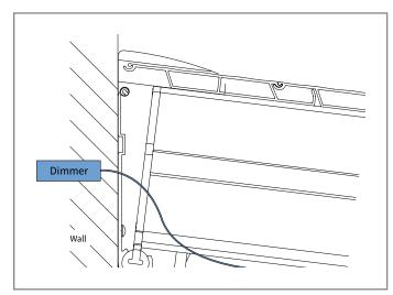
• Preferably run the wire through the wall before placing the dimmer.
