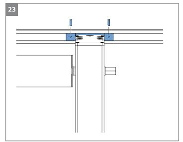
• Screw the connection pieces on the left- and right side to secure the center beam.
