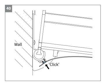
• Click the piping at the end of the fabric in the lower side of the wall profile.
