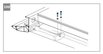
• Fixate the upright to the connection piece using two screws.
