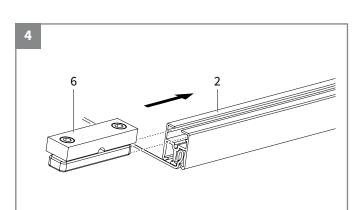
Slide the cord fixing block (6) in the front stiffener and place also precisely in the middle.
