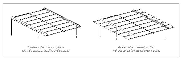
The side guides (1) are mounted against the outer veranda beams (A) in this manual. With a 4 meters veranda, the side guides (1) are mounted against the inner beams. This because the distance from side guide to side guide can be 3 meters maximum.
