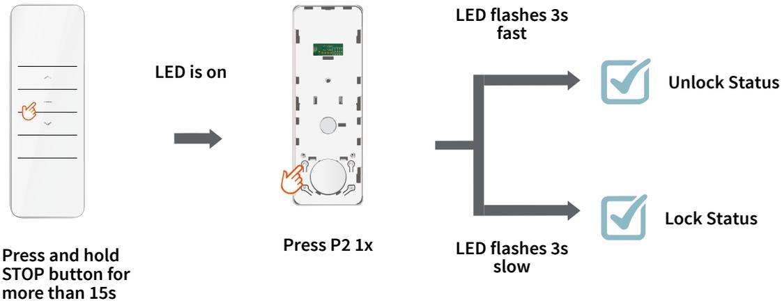
**Attention!** With the lock function you can not program functions in which you need two buttons like limit settings and change direction.
