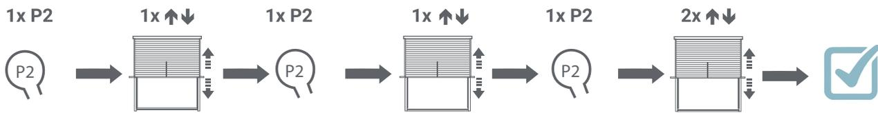
**Press 1x P2** of the existing channel. The product makes 1x up-down movement and/or beeps 1x.
