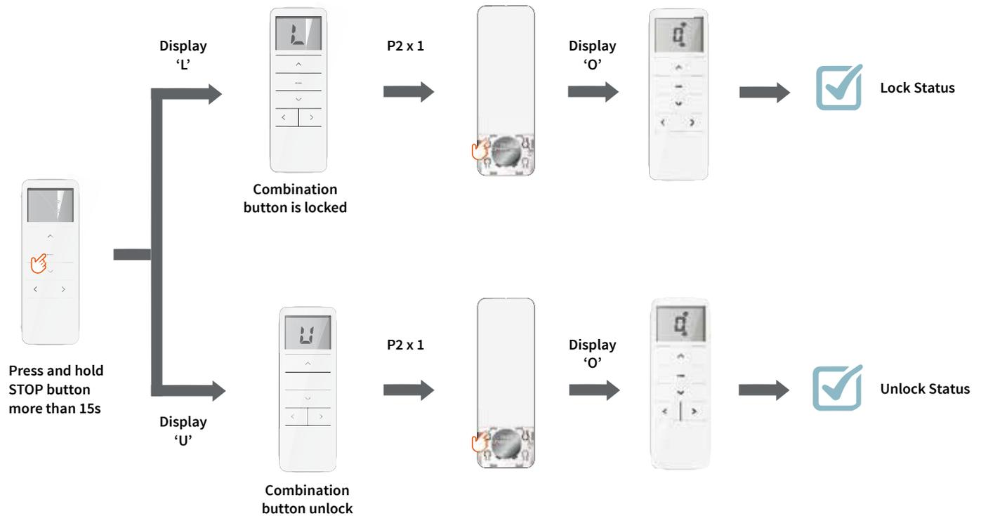
**Attention!** With the lock function you can not program functions in which you need two buttons like limit settings and change direction.
